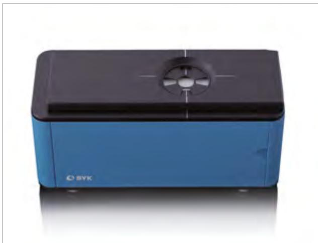
For repeatable results the product is placed into a sample drawer, which can be comfortably opened and closed. Magnets keep the drawer from sliding open. A mask is fit on top of the sample drawer to hold the spectro-guide in place and allow non-contact measurements of your products in a completely shielded compartment.
