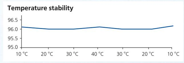
The micro-gloss gives the same measurement results between 10 °C–40 °C. No calibration or time for adjustment needed.
