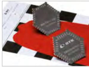
Wet film thickness measurement
