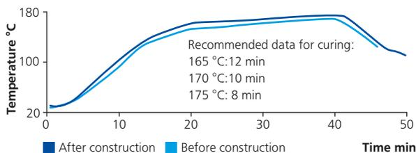
The paint manufacturer's recommended data for curing were as follows:
