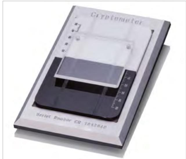
The value of the "wedge constant" of a top plate is the thickness in mils of the wedge of wet paint exactly over the demarcation line when the top plate is centered over this line and the scale reading is 25. Top plates with different wedge constants are included, depending on the opacity of the material to be tested:
