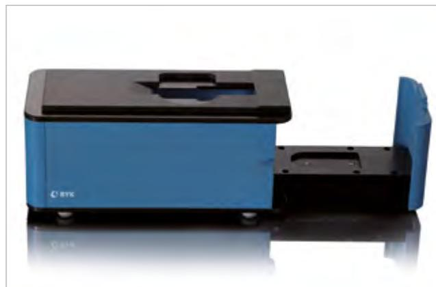
For repeatable results the product is placed into a sample drawer, which can be comfortably opened and closed. Magnets keep the drawer from sliding open. A mask is fit on top of the sample drawer to hold the BYK-mac i in place and allow non-contact measurements of your products in a completely shielded compartment.
