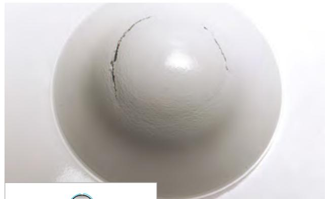
A die having a hardened and polished surface and a sample holder with a retaining ring are the heart of a cupping tester. The indenter that contracts the test panel is of hardened polished steel and forms a hemisphere of 20 mm ( 8 in ) diameter. The maximum cupping depth is approx. 14 mm. The test process is observed through a microscope or magnifying glass. When evaluating the test results, it must be carefully assessed when the coating system starts cracking.
