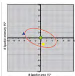
In order to set visually acceptable limits a new sparkle tolerance model was developed together with several partners from the automotive, pigment and paint industry. As a guideline the weighted total color difference equations were used resulting in an elliptical tolerance model.
