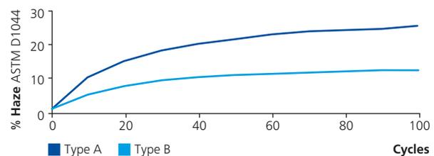
The graph above shows the abrasion results of different uncoated PMMA types used for public and sport glazing.
