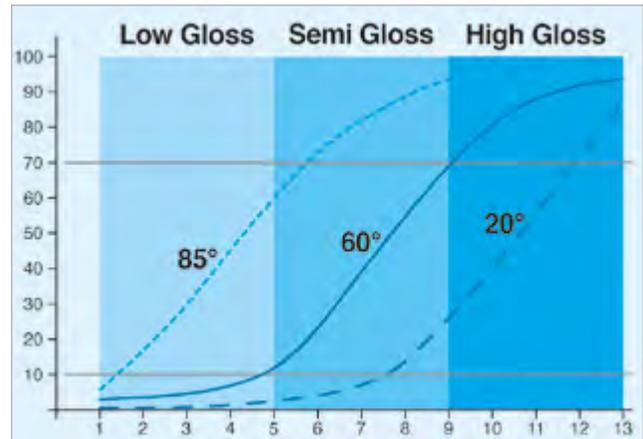
In this case study 13 samples were visually ranked from matte to high gloss and measured with the 3 specified geometries. In the steep slopes of the curves, the differences between the samples can be clearly measured, while in the flat part, the measurement geometry no longer correlates with the visual.
