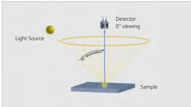
The 45/0 geometry simulates the normal condition used for color evaluation. For example, when we read a glossy magazine we position it to avoid the gloss from coming into our eye.
