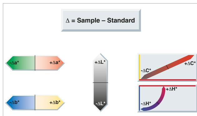
The color differences that can be accepted must be agreed upon between customer and supplier. These tolerances are dependent both on demands and technical capabilities.
