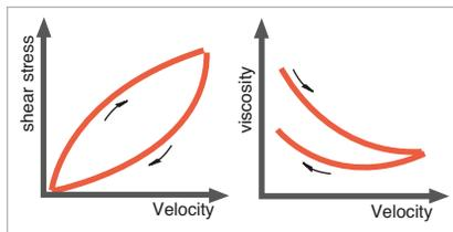
The viscosity of pseudoplastic materials will decrease with an increasing shear rate (shear thinning).
