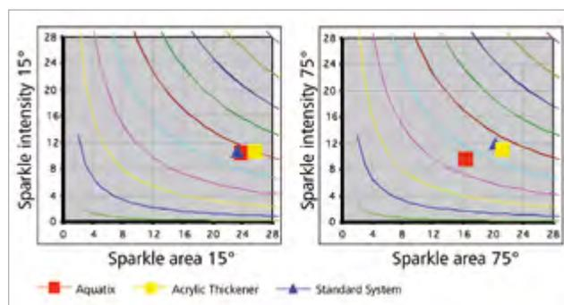
BYK-mac i measurement data correlates with a visual judgment. The sparkle area for the system with wax additive at 75° is smaller than for the two other systems. As Sparkle 75° evaluates flakes which are non-parallel oriented, this clearly shows that by using the BYK-Chemie wax additive AQUATIX® the orientation of the aluminum flakes is improved.
