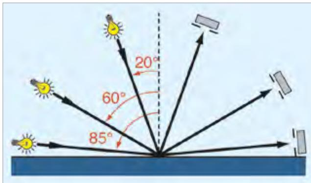
Glossmeters and their handling procedures had to be internationally specified to allow comparison of measurement values. The angle of illumination is of high influence. In order to obtain a clear differentiation over the complete measurement range from high gloss to matte, 3 different geometries, i.e. 3 different ranges, were defined:
