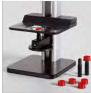
Sample pin for measuring e.g. distance sensor covers
