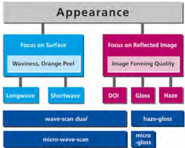
In order to guarantee reliable and practical quality assurance, it is necessary to define appearance with objective, measurable criteria. Accurate characterization of appearance does not only help to control quality, but improves quality and optimizes the manufacturing process.
