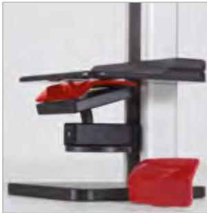
Flexible sample table for measuring e.g. headlamp cleaning device covers
