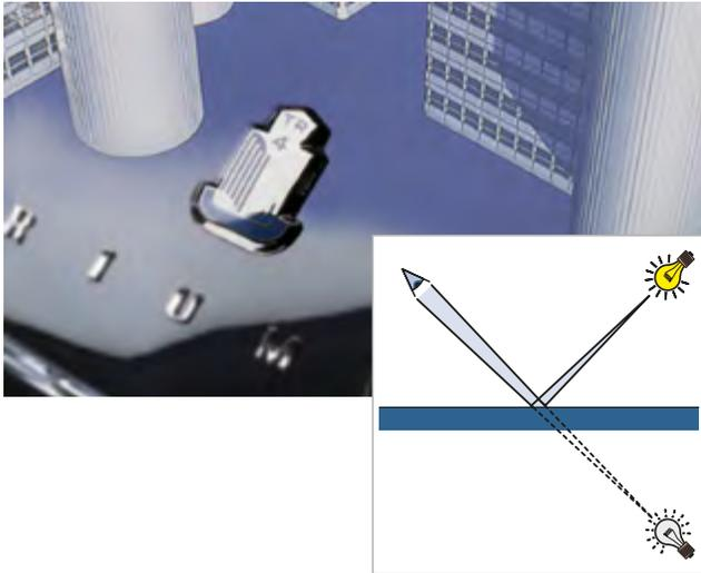
When we focus on the surface, we gain additional information about structure size and form. We see these structures as a wavy pattern of light and dark areas. This waviness is often referred to as orange peel or flow/leveling defects.
