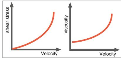
This behavior is known as “shear thickening”. When shear forces are applied, the liquid becomes more viscous.
