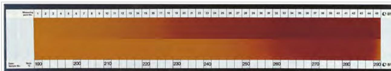
Whenever low temperature stable iron oxide pigments are used in baked coating systems or composite materials, it is very critical to define the production window in which the baking temperature will not affect the mechanical, chemical or the optical specifications.
