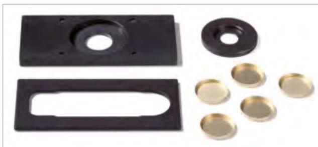
For repeatable results the product is pressed or poured into a sample cup. During sample preparation of pressed powders, it is important to always maintain the same plunger pressure as well as the same plunger tissue. It is recommended to use a fine-woven fabric to create a smooth, non-textured surface. The holder is equipped with a mask onto which the micro-gloss is placed for non-contact measurements.
