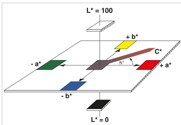
It consists of two axes  $a^*$  and  $b^*$  which are at right angles and represent the hue dimension or color. The third axis is the lightness  $L^*$ . It is perpendicular to the  $a^*b^*$  plane.
