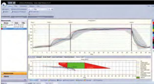
The temp-gard system controls the curing process and immediately evaluates the results. Within a few minutes all important information is available on the screen and can be printed out:
