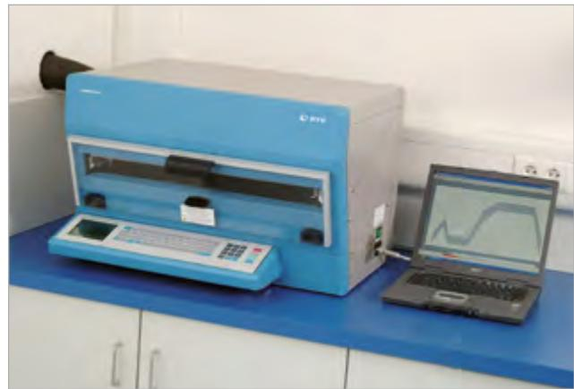
The gradient-oven helps to speed up R & D projects saving time and money. In QC testing of baked coating systems the gradient-oven produces repeatable results many times faster than using traditional convection ovens.
