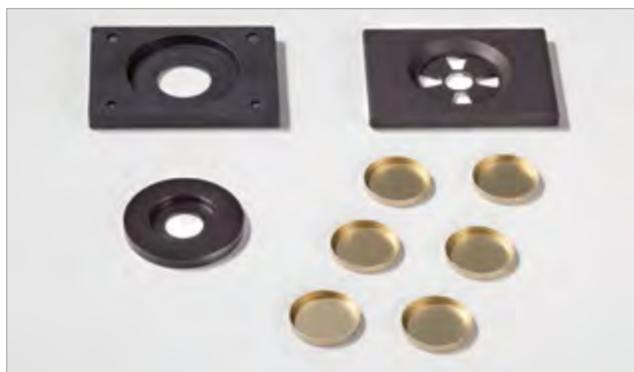
For repeatable results the product is pressed or poured into a sample cup. During sample preparation of pressed powders, it is important to always maintain the same plunger pressure as well as the same plunger tissue. It is recommended to use a fine-woven fabric to create a smooth, non-textured surface. The holder is equipped with a mask onto which the spectro-guide is placed for non-contact measurements.
