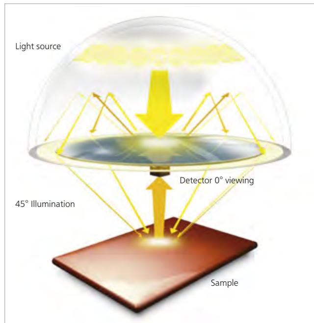
Measurement principle spectro-guide 45/0
