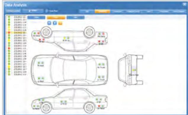
Additionally to the individual test results per check zone, the averages of groups (horizontals or verticals) are calculated and shown on top of the report. In case of color harmony analysis the difference of each check zone to the master standard and the differences between “panel matches” as defined in the organizer are displayed.
