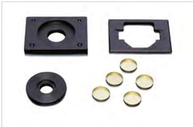
For repeatable results the product is pressed or poured into a sample cup. During sample preparation of pressed powders, it is important to always maintain the same plunger pressure as well as the same plunger tissue. It is recommended to use a fine-woven fabric to create a smooth, non-textured surface. The holder is equipped with a mask onto which the BYK-mac i is placed for non-contact measurements.
